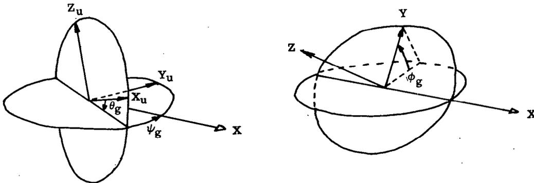
Figure 3.- Inertial axis system and body axis system.
