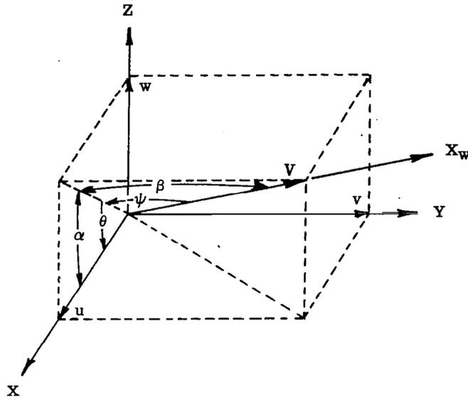
Figure 5.- Free-stream-velocity axis and body axis system.
