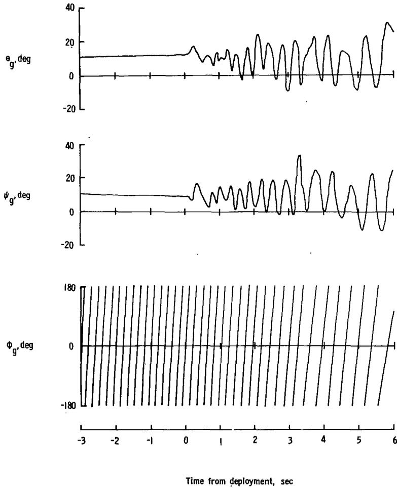
Figure 7.- Euler angles from gyro-platform data.
