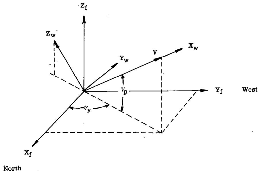
Figure 2.- Earth-fixed axis system and free-stream-velocity axis system.
